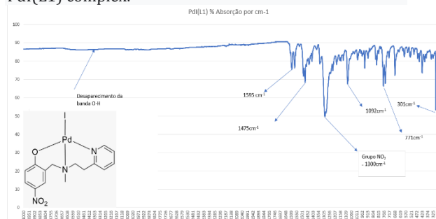
Fig. 7 - Infrared absorption spectrum in cm -1 for the PdI(L1) complex.
